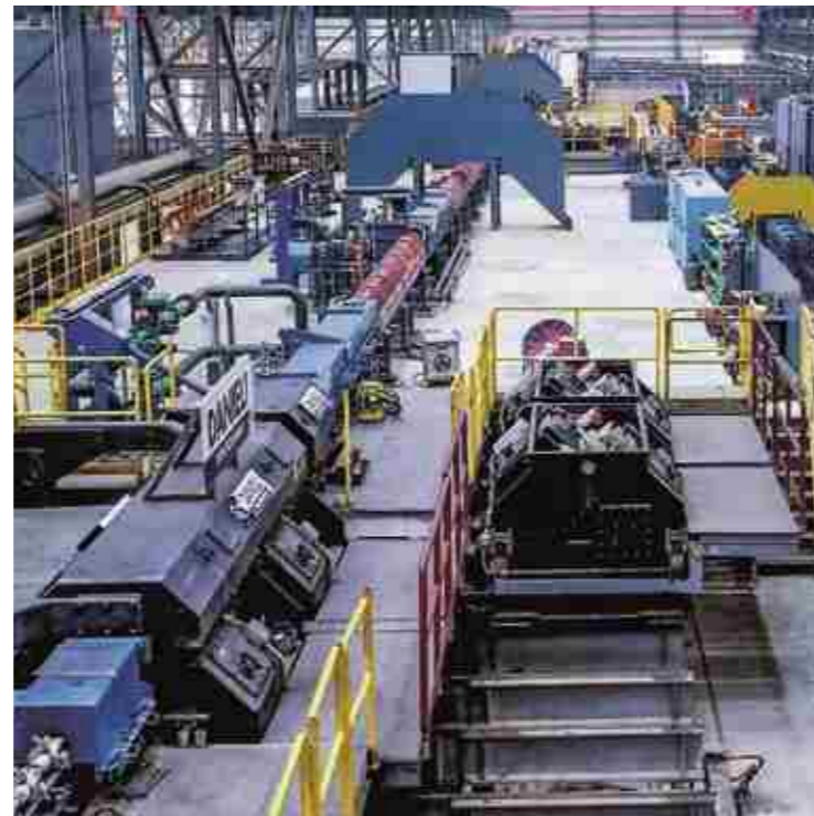
Fast-finishing block running at 105 m/sec
