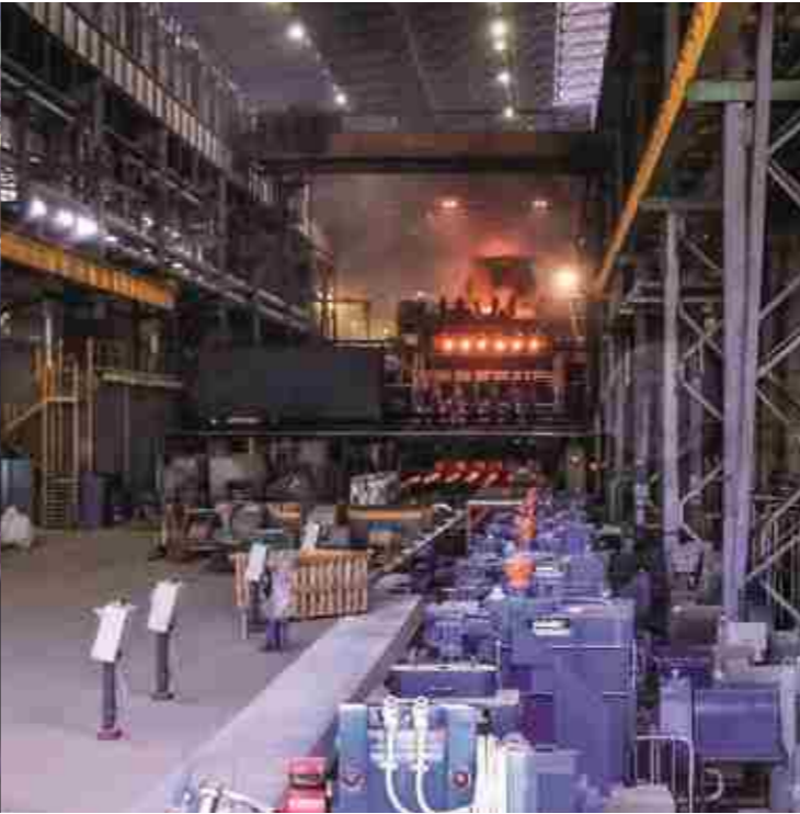
Six-strand FastCast caster equipped with FCC® and Power Mould®
