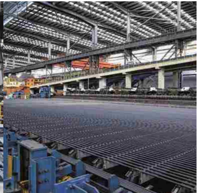
DRB - Direct Rolling and Bundling station
