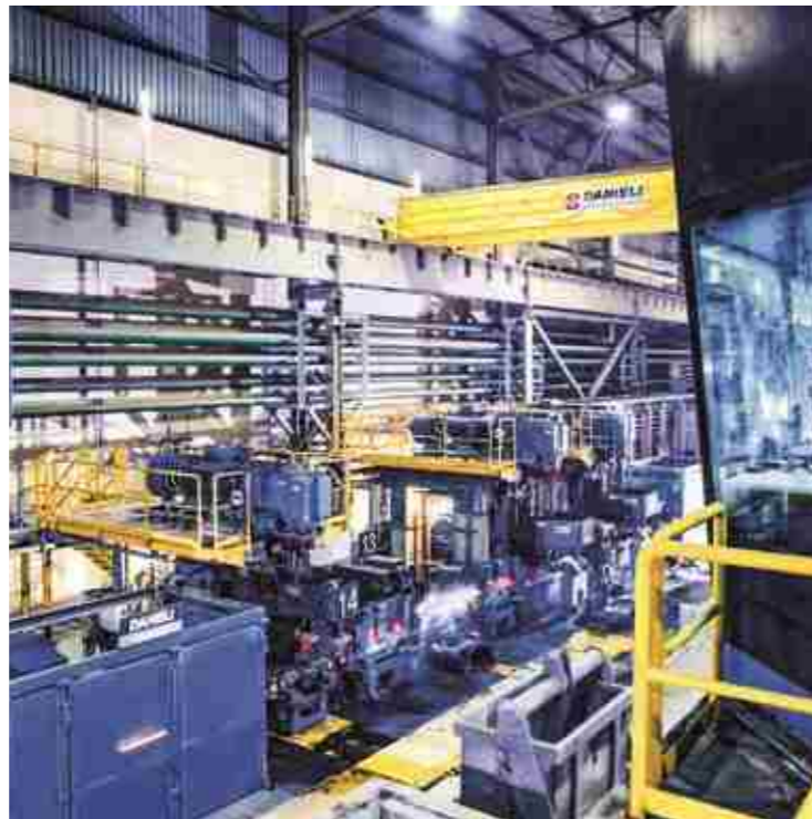
Six housingless-stand finishing mill
