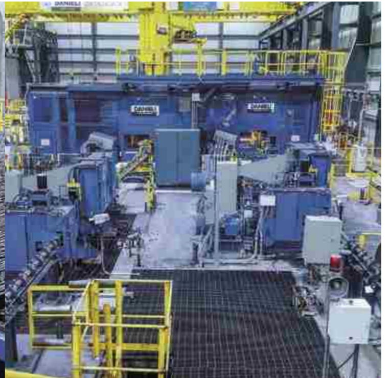
Twin bar-in-coil spooler line for coils up to 5 t
