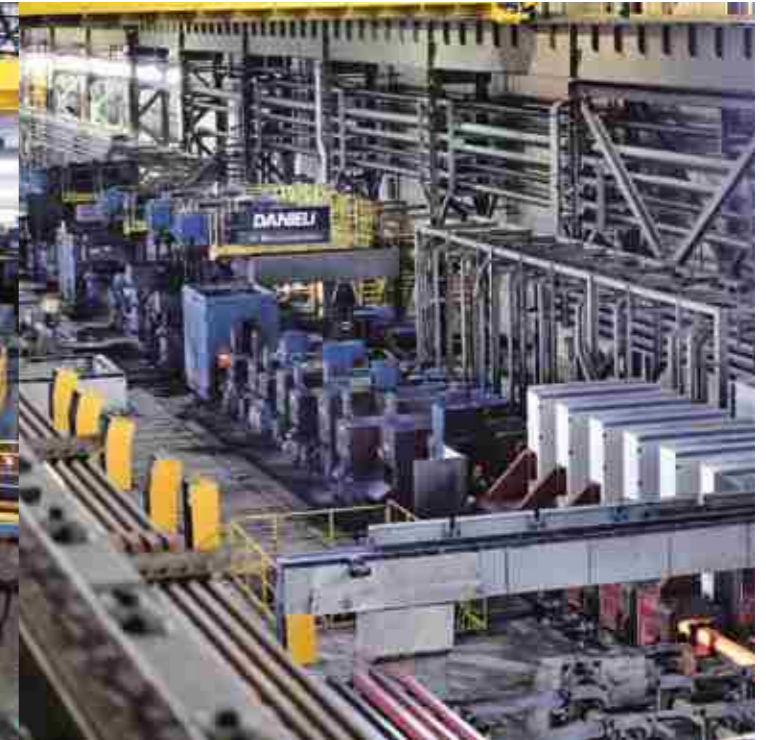
Endless casting and rolling line with Q-Heat inductors
