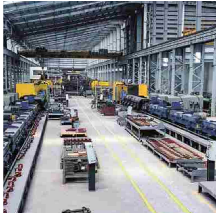
Twin-strand wirerod line with Fast-Finishing Blocks
