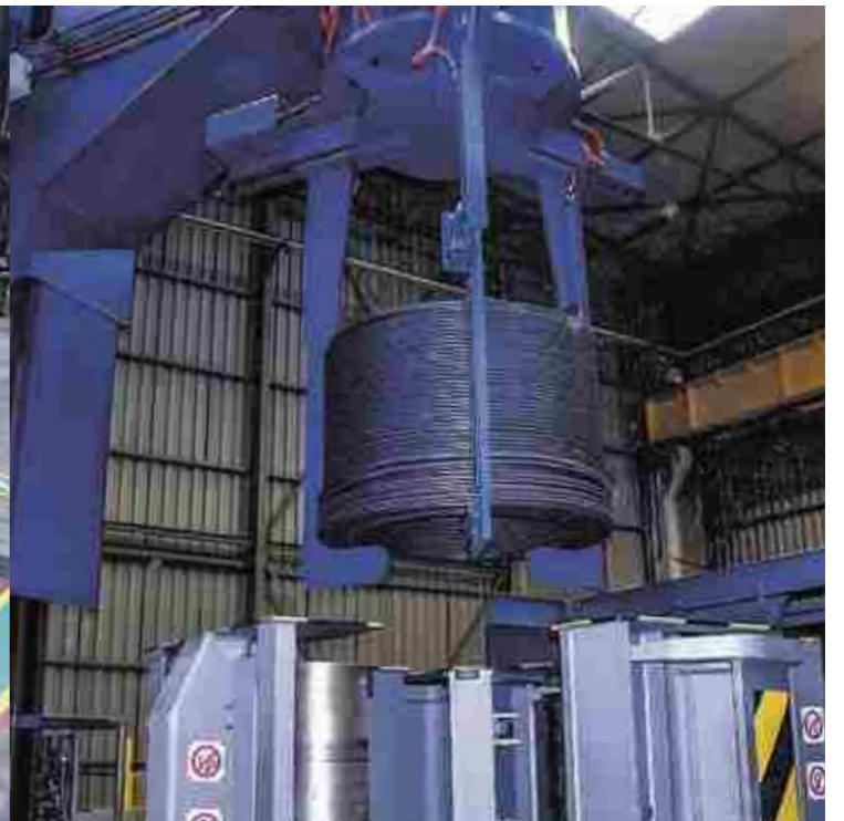
First 3-t coils spooled line operating in endless mode
