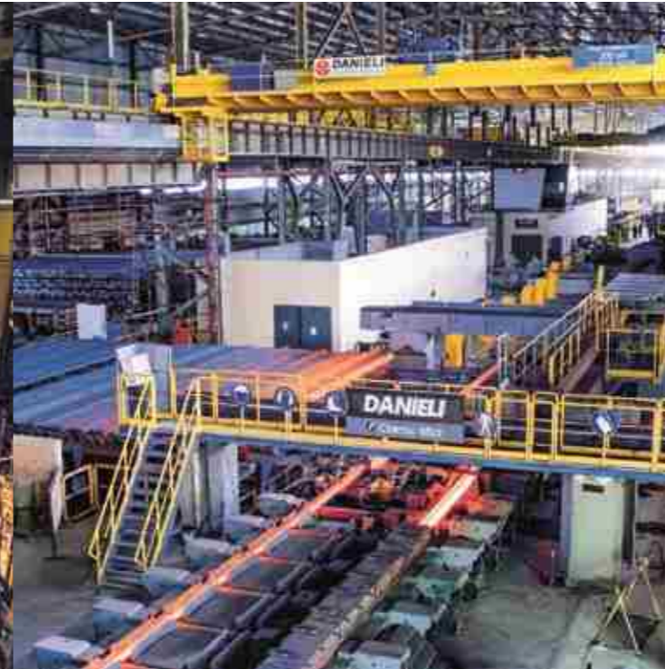
Three-strand billet caster featuring one FCC® for endless casting and rolling
