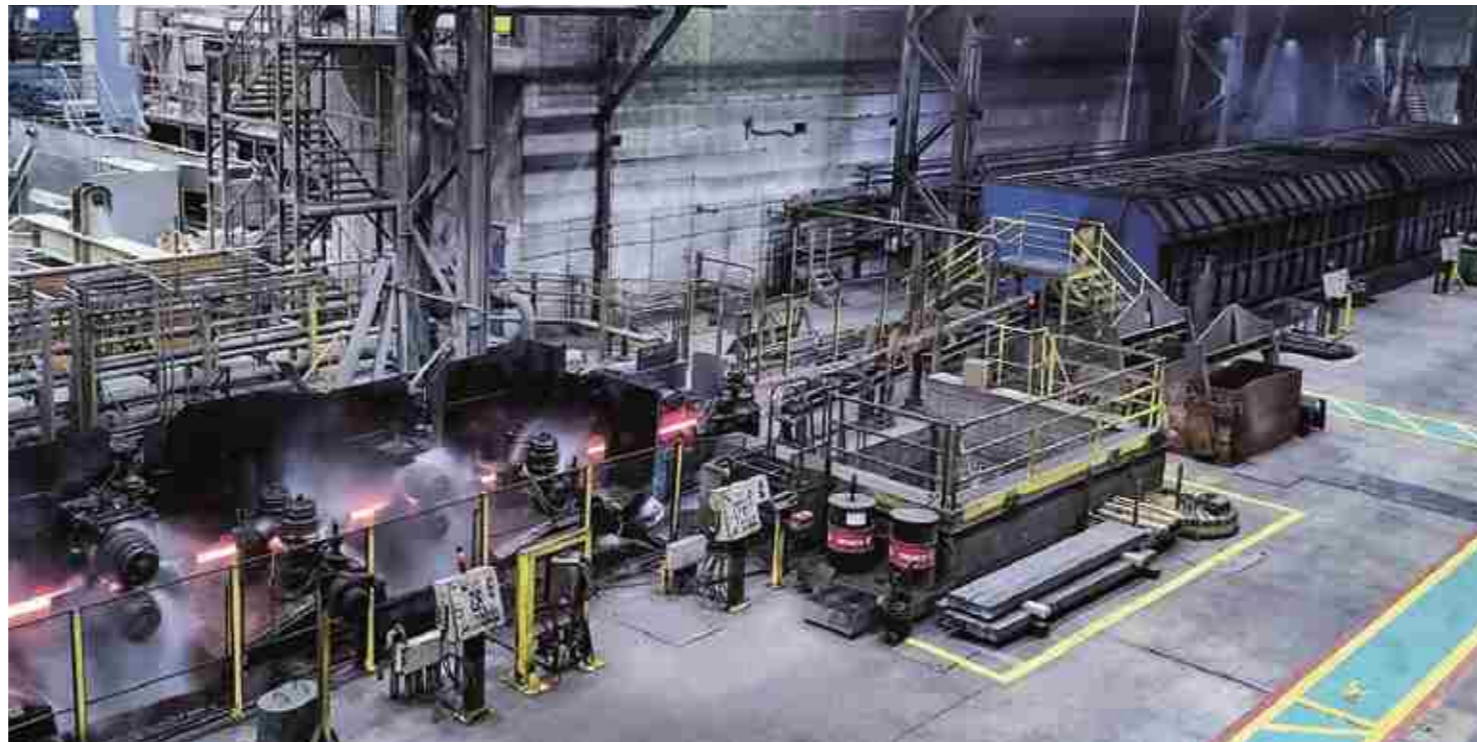
Roughing and intermediate mills with ESS energy-saving cantilever stands
