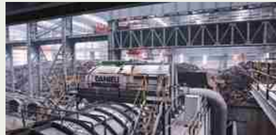
Zerobucket® continuous scrap charge
