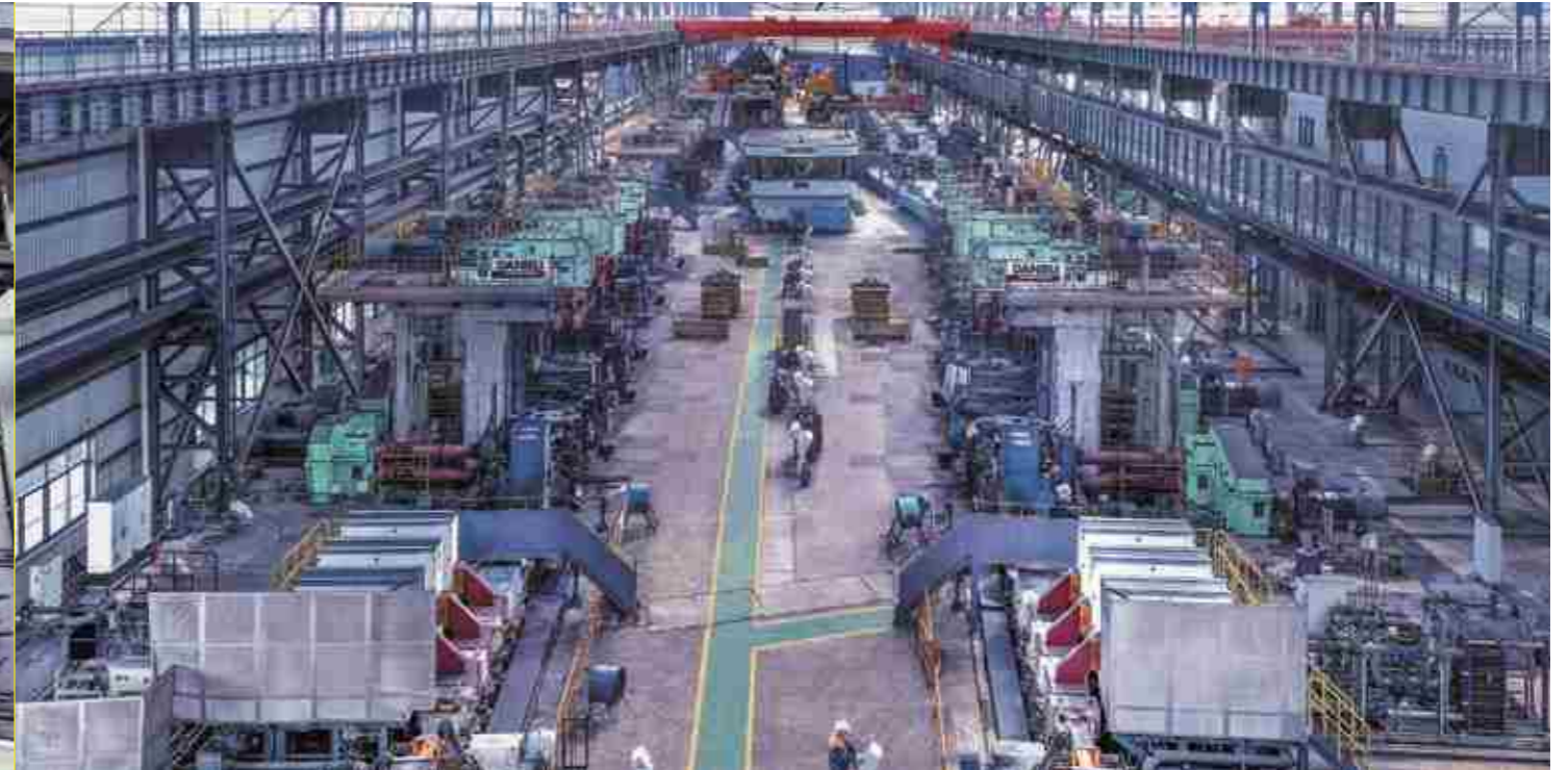
Twin rolling mill flexibly producing deformed bars and wirerod
